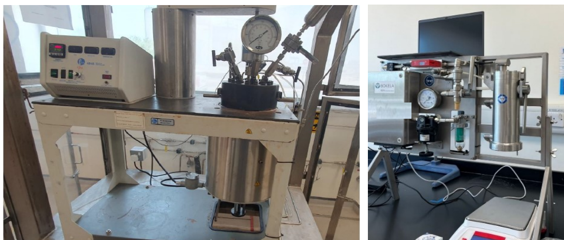
Figure 1. Laboratory equipment. Left: Parr reactor, Right: filtration unit.
